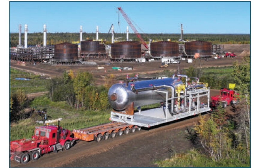
Inlet degasser at site
